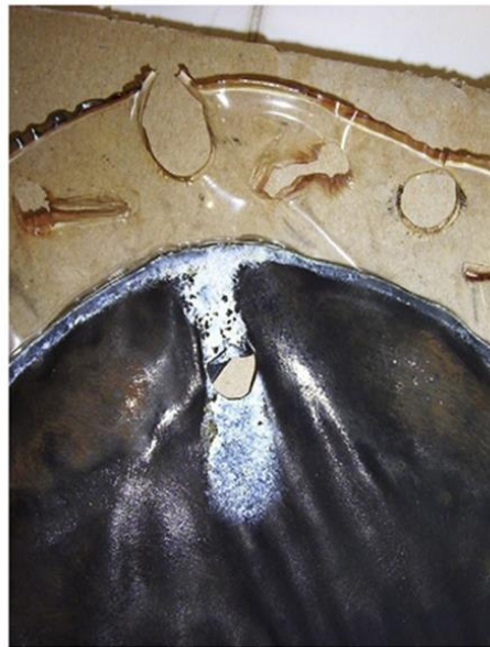
Figure 3: An extreme example of a hole present in a membrane post-operation. Reproduced with permission from [8].
