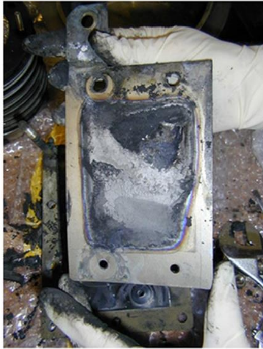
Figure 5: Bipolar/cell plate that has been damaged by a thermal event. Reproduced with permission from [8].
