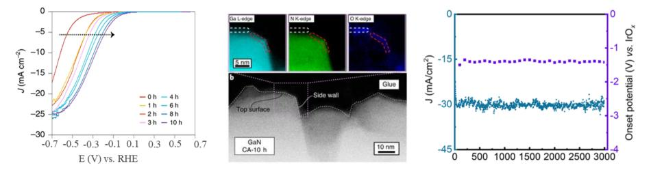
Performance improvement, instead of degradation, due to the formation of atomically thin GaON.
